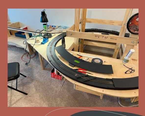
Inserting the Risers for the 5 1/2 loop Helix
