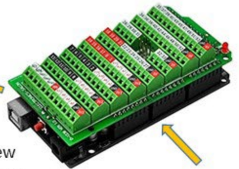
Arduino MEGA-2560 R3 (on bottom)
